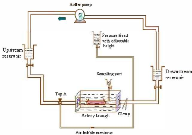
**Figure 1: Perfusion system used to impose laminar shear stress and hydrostatic pressure on aorta.**
