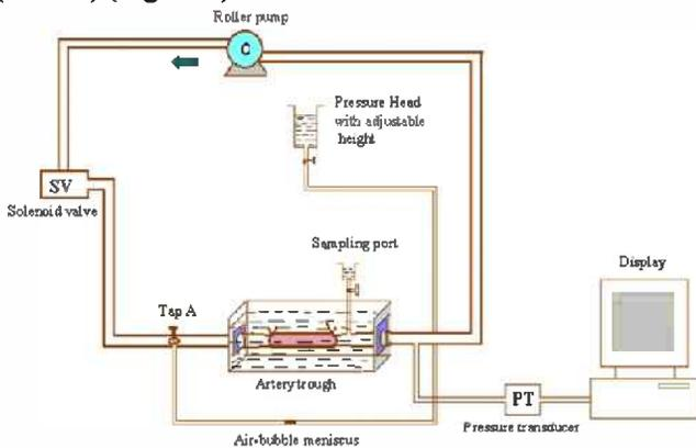
**Figure 2: Perfusion system used to impose pulsatile shear stress and hydrostatic pressure on aorta (catheter-tip pressure transducer inserted at the downstream end of vessel).**
